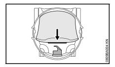
Push filter bag sleeve onto intake port as far as possible
