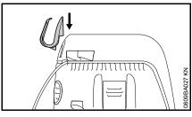
Attach holder for power cord on the right tab on the upper part of the vacuum cleaner
