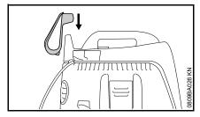
Connect holder for power cord via the support on the upper part of the vacuum cleaner
